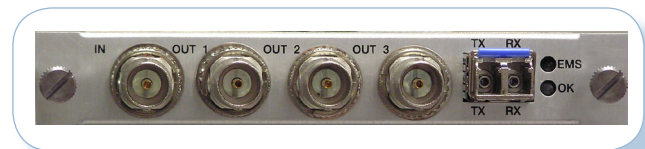
Rear panel includes one electrical Input, three electrical outputs, and SFP transceiver cage
